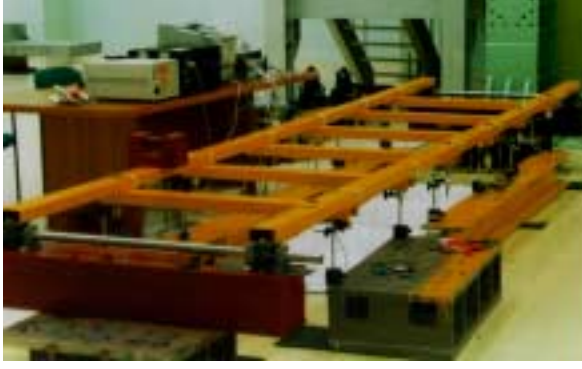
Figure 1: An overview of a grid-type bridge structure
