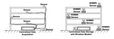
Figure 1 – Evolution from a Cable-Based to a Wireless Monitoring System
