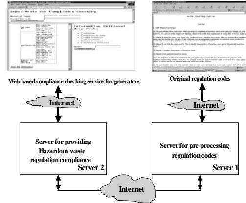
Figure 11. System architecture for the prototype system
