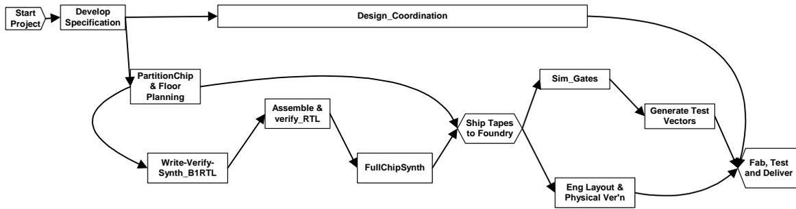
**Figure 11. Original CPM Diagram in Vite SimVision**
