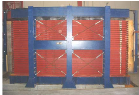
Figure 2: The UCSD medium size laminar box (Jakrapiyanun 2002).
