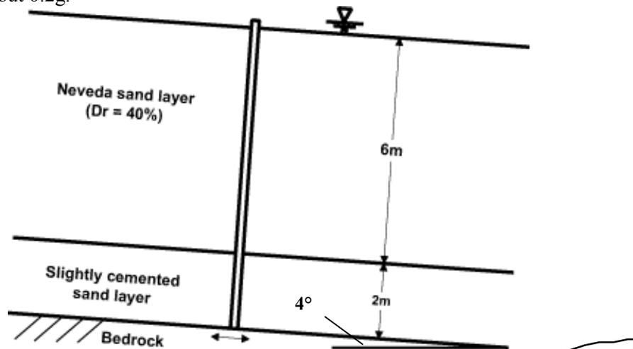
Fig. 3: A single pile foundation in a slightly sloping ground
