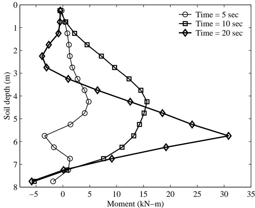
Fig. 11: Bending moment profiles at different times
