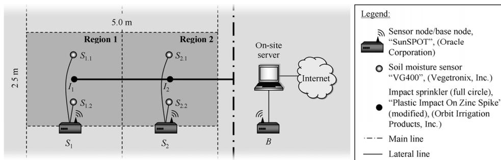
Figure 1. Schematic of the soil moisture monitoring system
