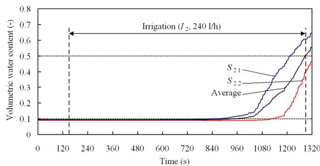
Figure 5. Average volumetric water content of region 2, calculated by the controller agent of sensor node  $S_2$
