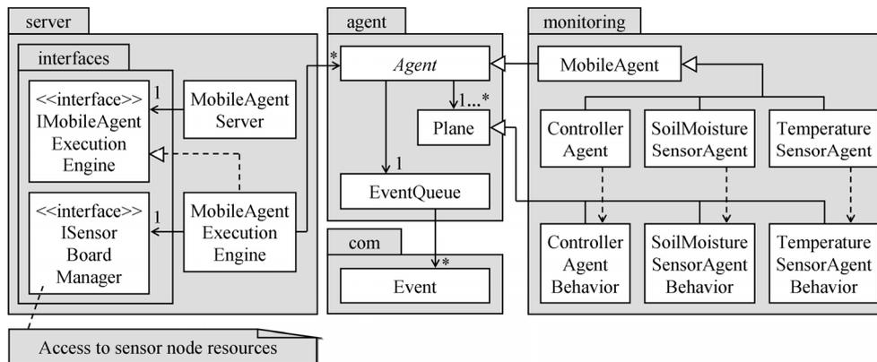
Figure 2. Abridged UML class diagram detailing relevant classes embedded in the wireless sensor nodes
