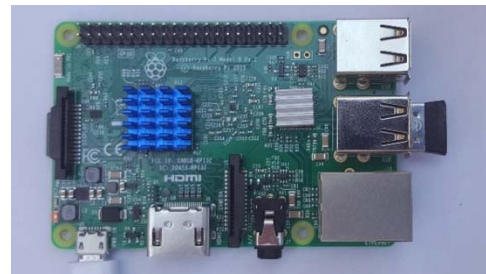
Figure 9. Raspberry Pi 3 Microcomputer running Python GPR scoring engine on Ubuntu 16.04. An additional heat sink (blue) was fitted to the CPU to allow it to operate at maximum capacity for a long duration of time.
