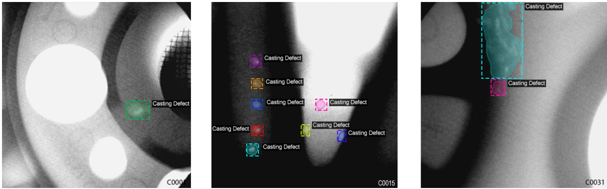
Fig. 14. Example detections of casting defects from the proposed defect detection system.
