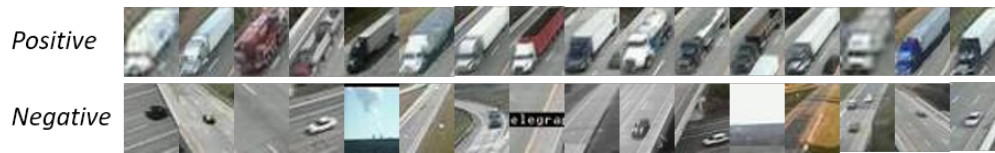
Figure 5. Positive samples (top) and negative samples (bottom) from traffic cameras.
