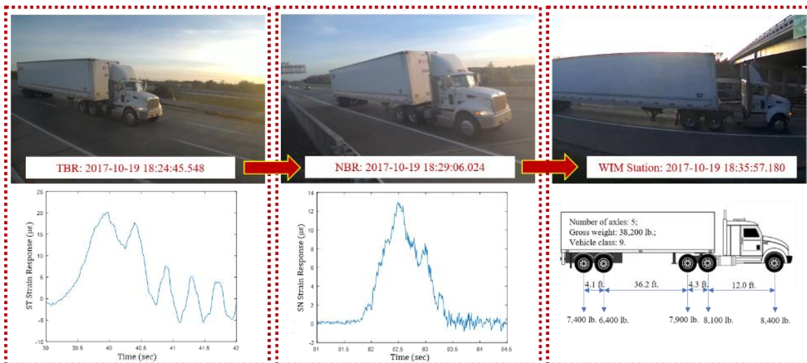
Figure 11. Example of integrated bridge response data and truck load weight data
