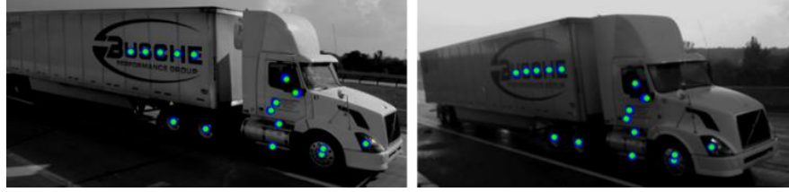
Figure 6. Same truck with top matched feature points highlighted by the MODS algorithm: (left) TRB and (right) NRB.
