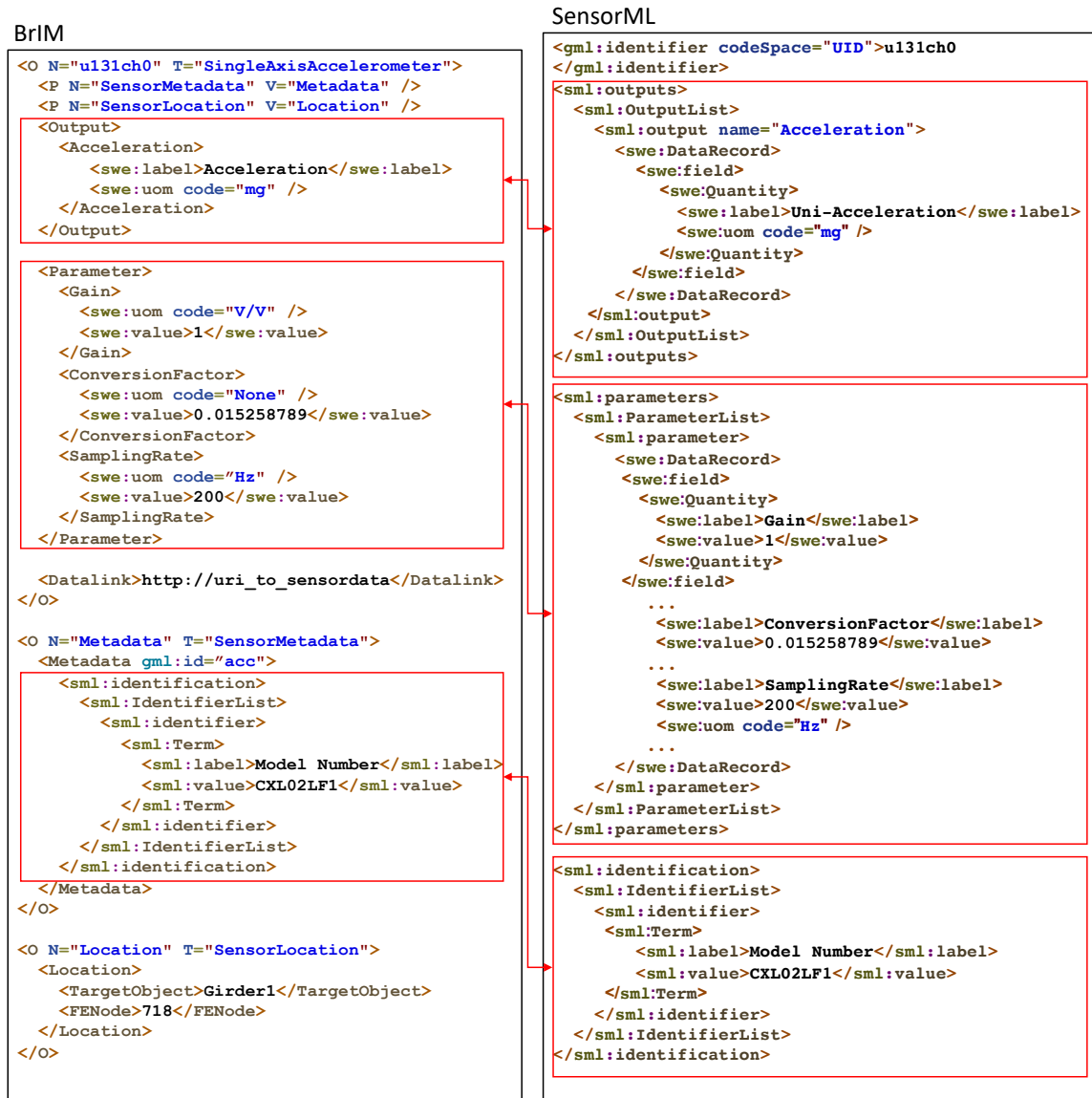
Figure 2.21 Sensor description represented using BrIM data schema and SensorML data schema
