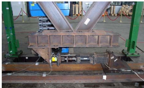
(a) MR damper installed between the 1st floor and the base floor
