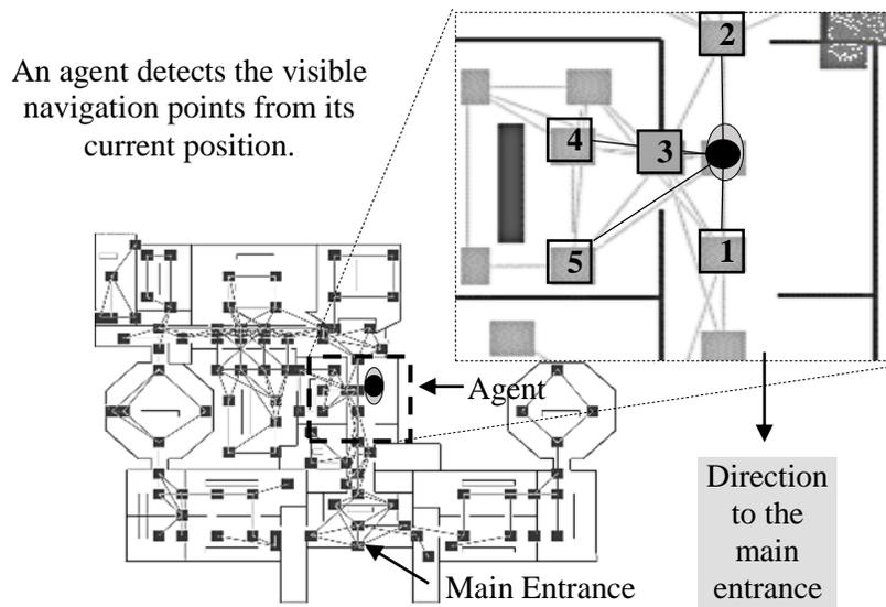
**Figure 3:** Illustration of visible navigation points given the agent's position
