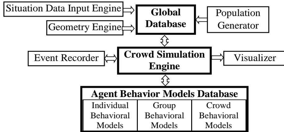
**Figure 1:** System architecture of SAFEgress
