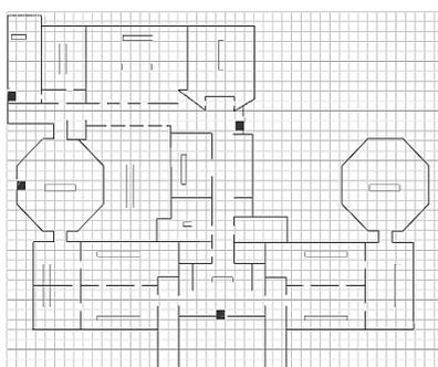
(a) Subdividing the space into square cells and initializing exits as navigation points
