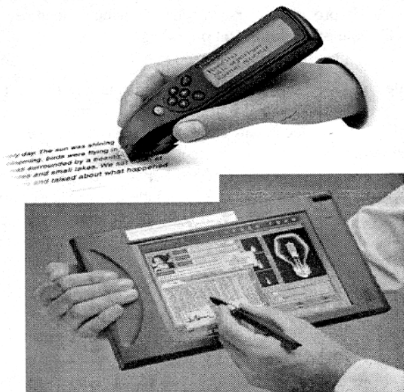
Fig. 3. Candidate appliances for mobile interaction with concept indexes: reading pens ( Quicktionary from WizCom Technologies Ltd., above) and book size computers with display tablets and pens ( Stylistic 2300 from Fujitsu Personal Systems Inc., below). (Pictures obtained from manufacturers' Web site and reproduced with their permission.)
